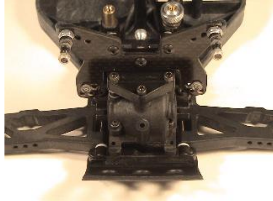
Picture 8: Front Shock Tower installed.
