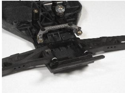
Picture 5: Complete Servo Saver (Bell-Crank system) and Tie Bar Installed.
