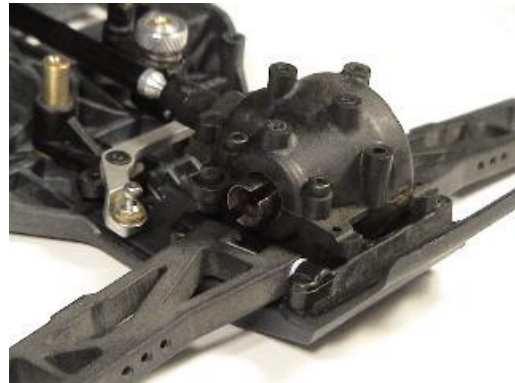
Picture 6: Gear box installed in the front end.
